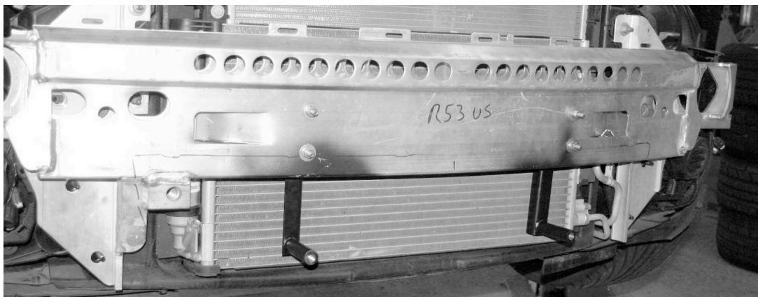
Bumper beam and struts in place and ready for bumper skin
