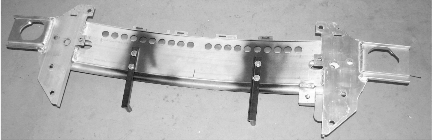
Struts shown bolted to back side of bumper beam after aligning with bumper cover
