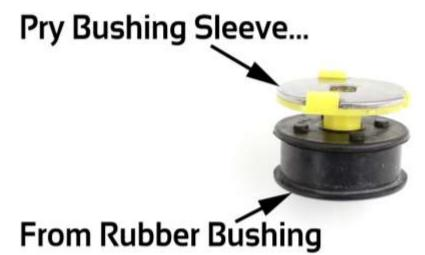
14) Remove plastic bushing sleeve from rubber bushing by carefully prying between each piece, working from one side to the other with a flat head screw driver.
