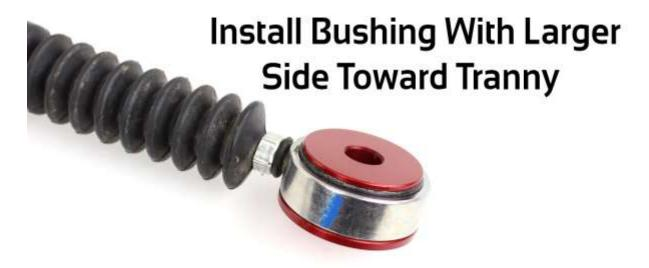
16) Apply grease to outer portion of yellow plastic bushing sleeve and to inside of ALTA Shifter bushing. Snap bushing sleeve into ALTA shifter bushing until it snaps into bottom of bushing. If installed correctly, OEM sleeve should spin freely in ALTA Bushing.
