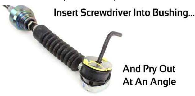
13) With cable free, insert screw driver (or any small tool) into hole of shifter bushing, and pry bushing from cable. **NOTE: Take** extreme care not to bend cable beyond the angle as shown, or damage may occur.
