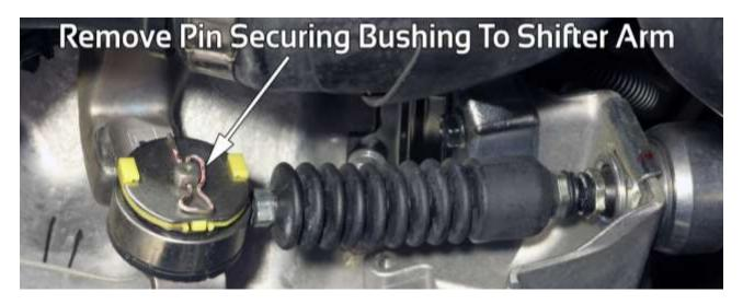
12) Locate and remove small pin/clip securing larger bushing to pivot. Pull up slightly to free from shifter mechanism and lift shifter cable from bracket and pivot. NOTE: Potential shifter cable damage can occur if cables are pulled up too far or angle too far from center. See the picture above showing the limited angle that can be had from the cable. Take great care not to force the cables in the wrong direction over the next few steps.
