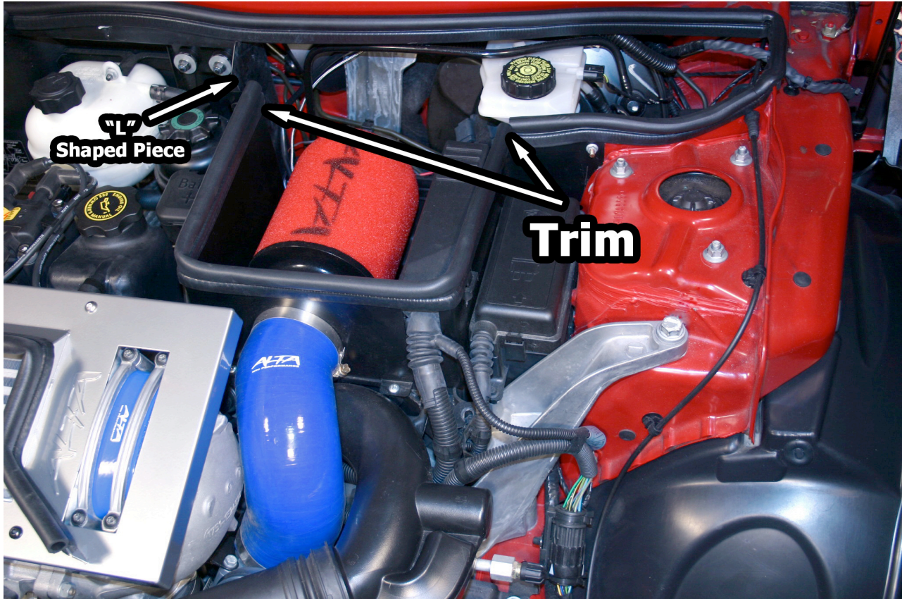
Completed Install: Note trim around box and wall removed (optional Silicone inlet hose shown)
