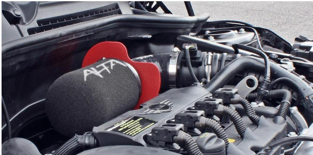
16. We highly recommend that you modify or remove the OEM hood scoop plug to direct fresh air at your ALTA intake. You can skip this step if you have small holes in your hood scoop (most 08+ cars have this). If yours is blocked off, we feel this is a necessary step.
