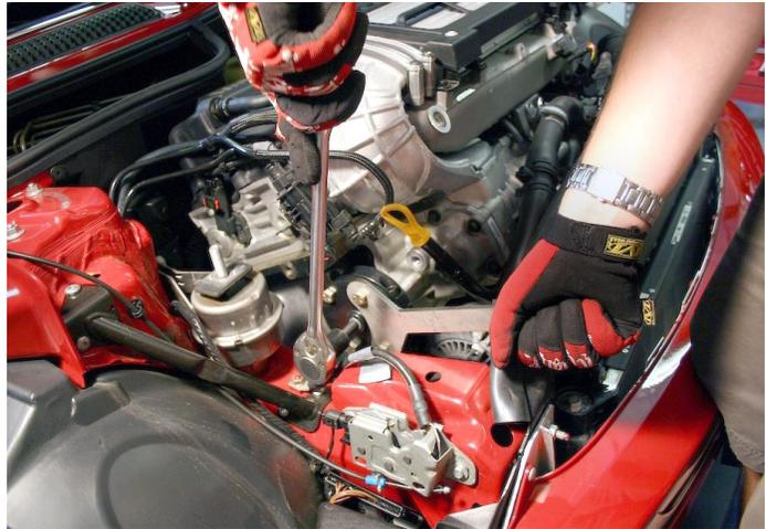
18) Install ALTA Supercharger pulley to supercharger shaft according to above instructions. Picture below shows pulley completely installed onto supercharger shaft.
