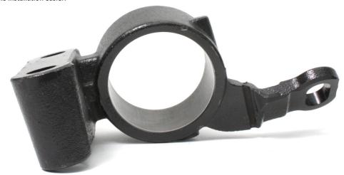
7) The ALTA PSRS can be pressed into the mount in many ways. See below pics demonstrating the different effects. Once you have determined where you want to press the PSRS into the set PSRS with logo facing the front of the car, and press completely into bushing mount. It is important to press on the body of the PSRS not bushings.
